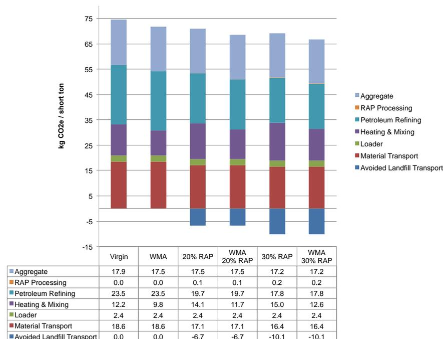
Figure 2: Difference in GHG intensity Virgin materials vs. RAP/WMA (WMA) asphalt mixes.
